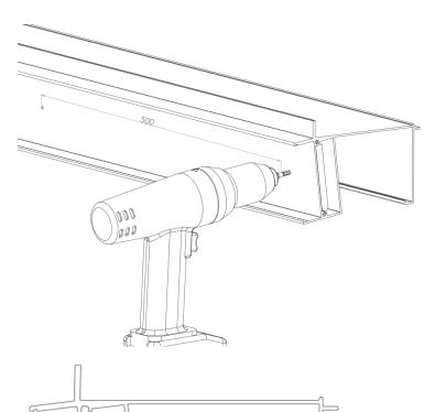
Pre-drill a 3mm hole through the back of the gutter into the steel bar at approx. 500mm intervals along the length of the gutter. Be careful not to pierce the inside wall of the gutter.
