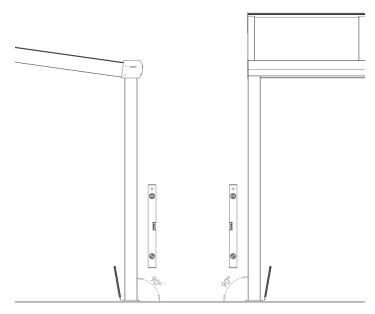
Once the roof beams are installed, check again that the veranda is installed at 90 degrees to the wall using a laser, or large set square. Then, using a spirit level check that the posts are vertical in both directions.
