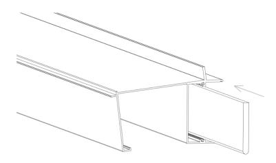
Slide the steel bar into the cavity at the back of the gutter.
