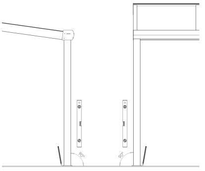
**Surface mounting**Mark outside edge of base platform position
