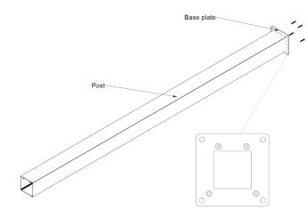
c) Fix standard base plates – if surface mounting with standard base plates or securing below ground.
