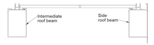
The glass should be pushed against the wall profile so that it overhangs into the gutter by approx. 50mm
